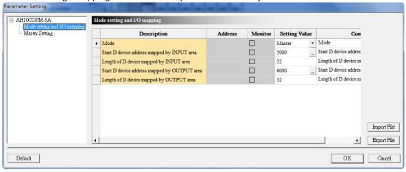
AH10COPM-5A functions as a master station. If the start input address set is D5000, and the start output address set is D6000, the mapping areas assigned will be as described below. The data lengths that the users can set must be in the range of 0 words to 480 words.
