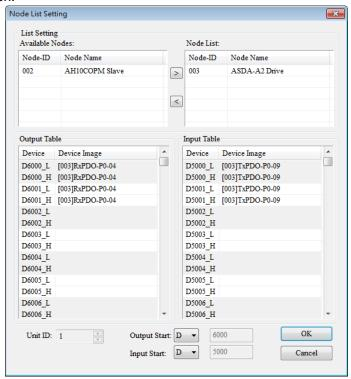
The users can add node ID 2 to the list under **Node List** in the same way. When node ID 2 on the list under **Node List** is selected, the data registers in the AH500 series module onto which the I/O data in node ID 2 is mapped are shown in the **Output Table** section and the **Input Table** section.
