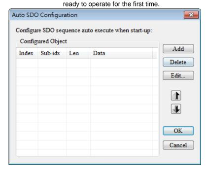
After the users click **Add**, the **Add New SDO** window will appear. The index in the **Index (hex)** box is the index of the parameter which will be accessed, and the subindex in the **Sub-Index (hex)** box is the subindex of the parameter which will be accessed. The length in the **Length (dec)** box is determined by the data type of the parameter which will be
