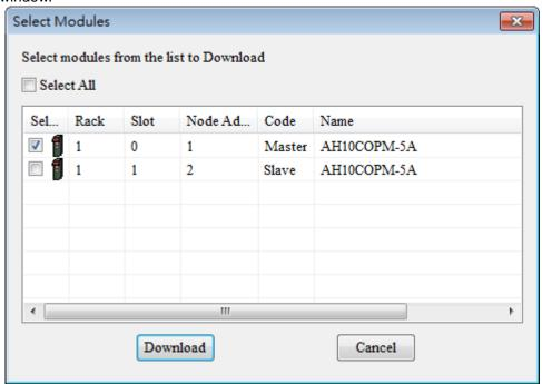
After the users click **Download**, the configuration data set will be downloaded to the AH10COPM-5A module selected. If the AH10COPM-5A module is operating, the users will be asked to stop the AH10COPM-5A module before the configuration data is downloaded.
