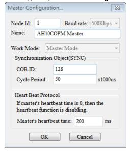
COB-ID: Setting the COB-ID used to send synchronous messages
