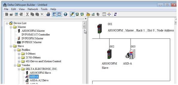
Setting the parameters in the master station on a CANopen network
